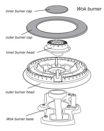
When reassembling the Wok burner, turn over the large base ring and find the 'D' shaped area.
